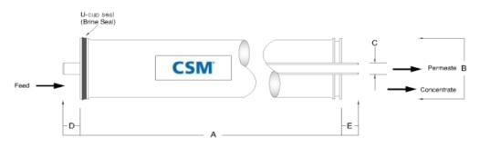
1. Each membrane element supplied with one brine seal, one interconnector (coupler) and four o-rings. 2. All NE4040 elements fit nominal 4.0 inch (101.6 mm) I.D. pressure vessels.
